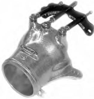
The R&D VTS/Auto Drop Nozzle is the first manually activated VTS nozzle with Auto Drop functions! When riding with the VTS adjusted in the neutral position the nozzle will drop 5 degrees in the turns allowing for a much smoother high speed turn to be made. When the steering reaches the straight position the nozzle returns back to the straight position. When riding with a full tank the best VTS setting is usually in the
