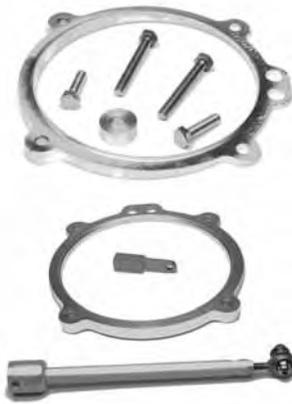
4-TEC doesn't have a trim system is a mystery. Extensive testing has led our development team to wedge the reduction nozzle up 2.5 degrees which will inexpensively give your 4-TEC better handling everywhere and provide a boost of 1 to 2 mph in top speed performance. The billet aluminum CNC machined 2.5 degree reduction nozzle wedge kit was designed to work with the OEM O.P.A.S. system and installs easily in 15 to 20 minutes with R&D's "easy install" directions.
