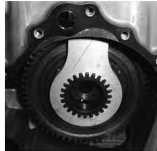
This R&D tool enables the clutch to be changed in a matter of only minutes. With the supercharger and front engine cover removed the tool drops down through the case and secures the drive gear at the front of the crankshaft from rotating when the
