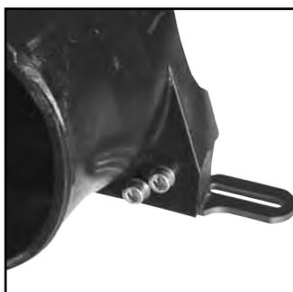
This quick steering adapter fits the stock superjet nozzle. It will give you the option to play with the quickness of the steering from really aggressive to really smooth. It will also give you a lot more turning ratio for free style. RRP quick steering adapters are black.
