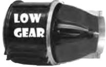
In low gear the shuttle lets a large volume of water be moved to accelerate the craft.
