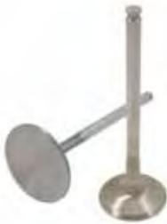
RIVA High Performance Valve Kits are engineered to improve reliability and performance in high-boost supercharged & turbocharged engines. Intake valves are built from high grade EV-8 (24-4N) stainless that is extremely resistant to corrosion. Exhaust valves are built from inconel alloy (IN-751) that is highly resistant to heat
