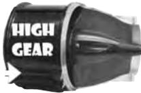
As speed and pump pressure increase, the shuttle is forced out into the exit nozzle, reducing its size and increasing water velocity. This increases top speed.
