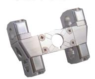
The Speed Magic "X-Mount" for the RXP-X and RXT-X improves handling by lowering the steering head 85mm lower than the stock position and moves the rider forward for a more aggressive riding position. Accepts standard 7/8" (22.2mm) handlebars.
